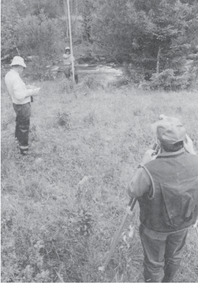
Figure 49. Good location for level setup.
