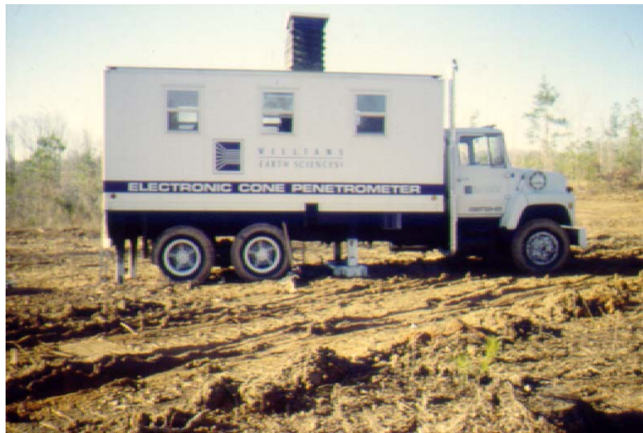
Figure 13. Cone penetration testing from cone truck.
