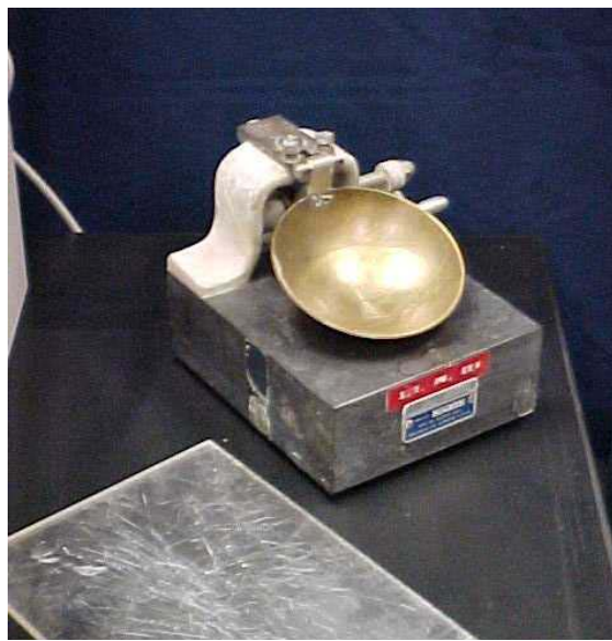
Figure 24. Equipment used for Atterberg limits testing of soil.
