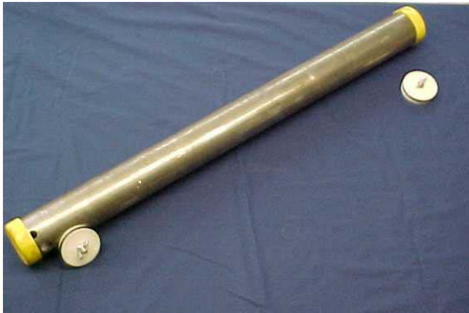
Figure 5. Thin walled (Shelby) tube for sampling (with end caps).
