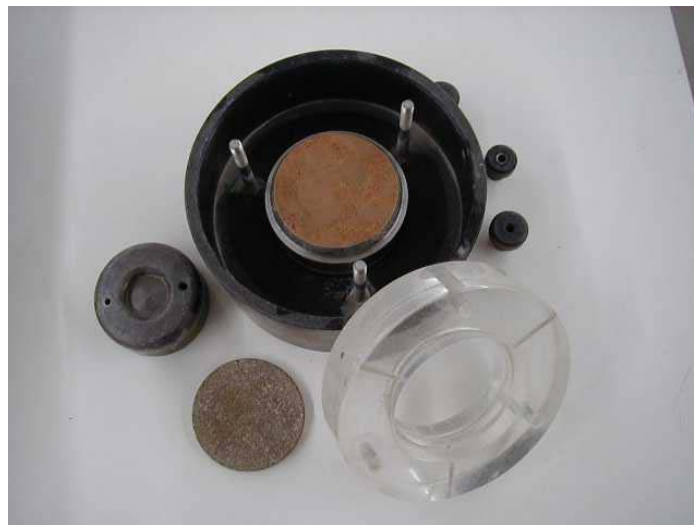
Figure 26. Components of consolidation test (photograph courtesy of GeoTesting Express).
