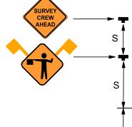
When surveying on road having edgelines or when 10 ft. of driving surface cannot be maintained, one lane shall be closed. Refer to appropriate lane closure typical applications.
