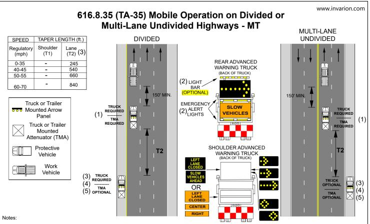
A protective vehicle occupying any portion of a lane shall be equipped with a flashing arrow panel and a TMA.
