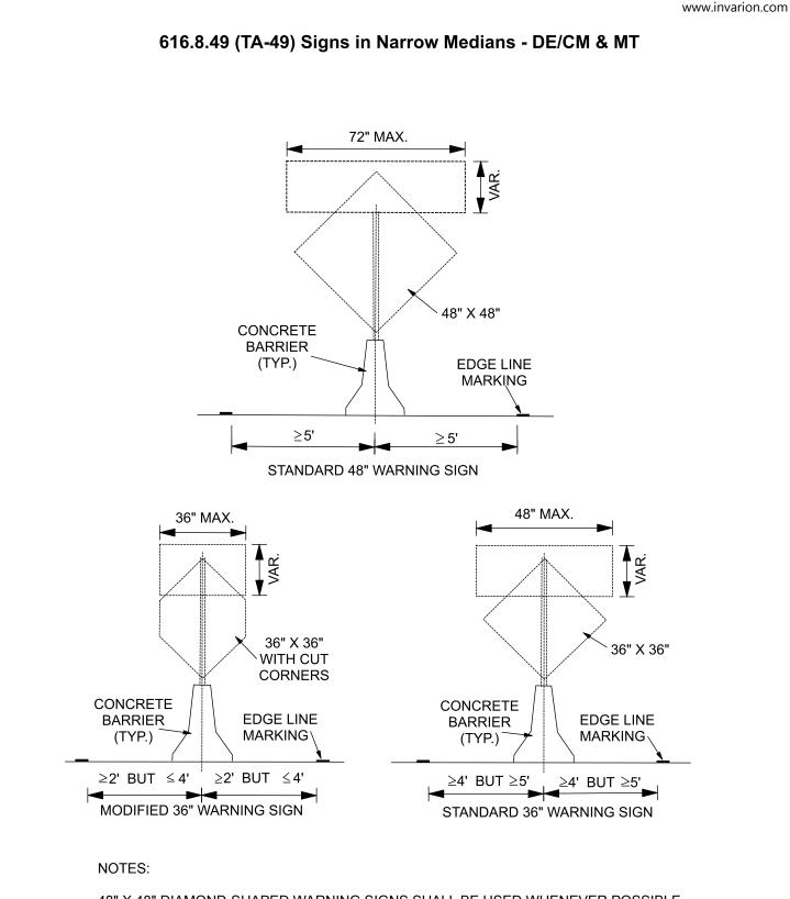
48" X 48" DIAMOND-SHAPED WARNING SIGNS SHALL BE USED WHENEVER POSSIBLE. RECTANGULAR SIGNS SHALL NOT BE USED IN LIEU OF DIAMOND-SHAPED WARNING SIGNS.
